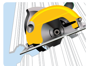
Sawing the panels Figure 4
